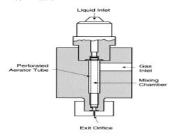
Fig: 1. A typical effervescent atomizer [1]
