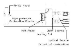
Fig: 4. Combustion Chamber
