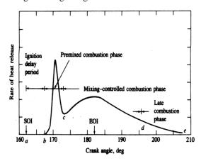
Fig: 2. ROHR Curve for Diesel Engine [3]
